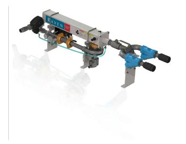
The AccuFlow<sup>™</sup> anhydrous ammonia (NH3) distribution system converts NH3 gas to liquid, keeping it cold and fluid during application. With fast cooling, high capacity, and application rates up to 80 gallons per minute (gpm), you can cover more acres per day. AccuFlow is a more accurate and efficient replacement for dual cooler systems.
