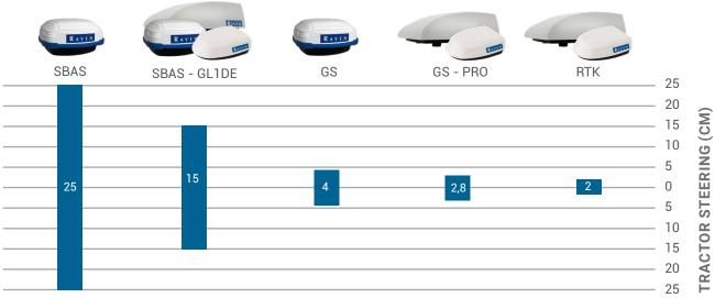
NOTE: Achievable accuracy and convergence time may vary based on capability of receiver, antenna, ionospheric activity, and multipath environment
